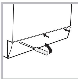
1. using a screwdriver, remove the cover panel on the lower front part of the washing machine (see figure);
